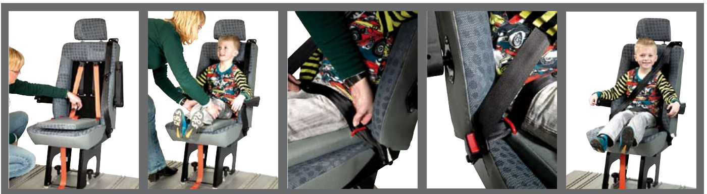
Children in Group 3 are secured by means of the built-in 3-point belt. The belt should pass under the red hooks on either side of the child's hips
